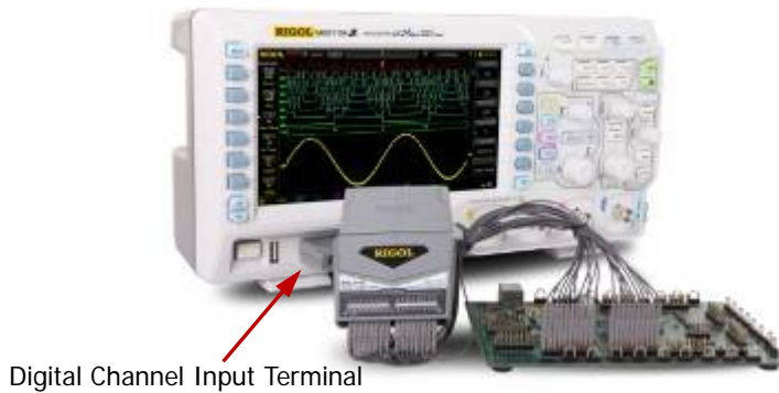
Figure 1-6 To Connect the Logic Probe
